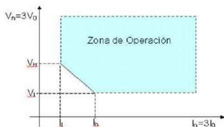
In this characteristic the values for  $I_1$  and for  $V_h$  are the ones given for  $I_{ns}$  and  $V_n$ . The typical values for  $I_h$  and  $V_l$  are:  $I_h = 3 \cdot I_1$  y  $V_l = 2,2 \text{ V}$  ( $U_r = 110/3$ ).
