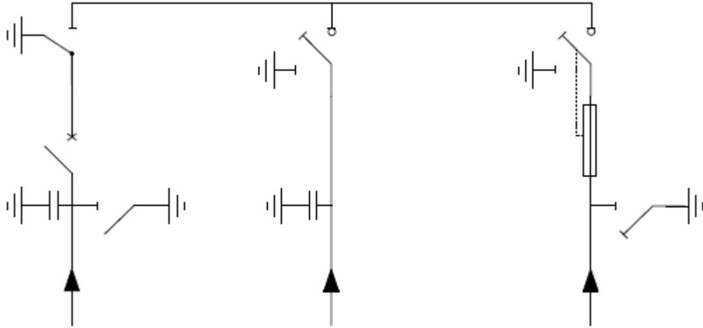
Figure 2: MV section using circuit-breakers
