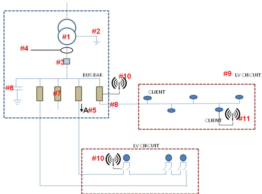
**Figure 15: Support Scheme for LV Grid protection**
