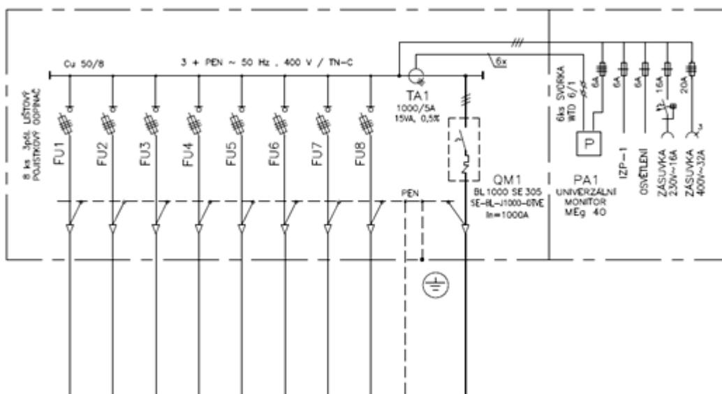
Figure 8: LV section using fuses protection
