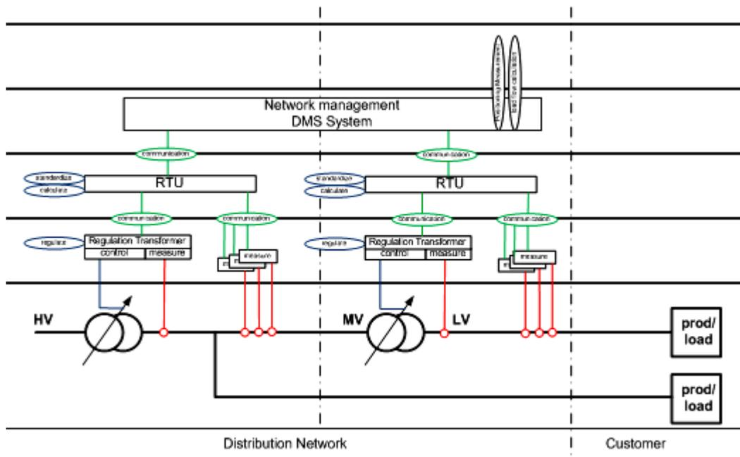
**Figure 4: Voltage regulation and flow control in the distribution network**
