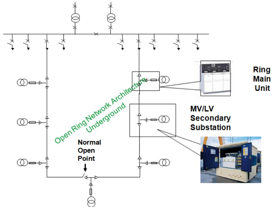
The RMU can have one or two power transformers, protected by switch-fuses..
