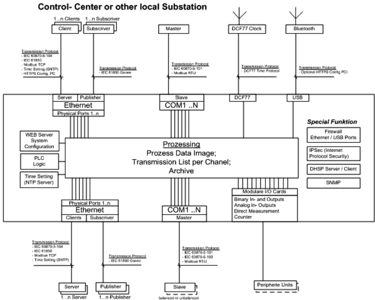
Figure 3: Network topology and block diagram of a RTU
