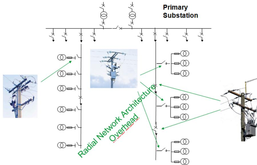
This circuit consists of a main line and many different secondary lines, which normally end in one or several overhead MV/LV transformer substations (OTS).
