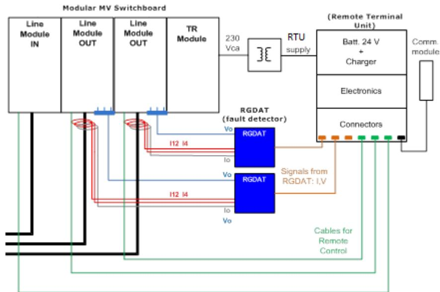
Figure 12: Standardized architecture of a remote controlled and automated secondary substation applied in Italy and Romania
