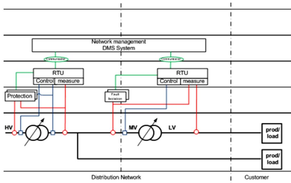
Figure 5: Connection and disconnection of network equipment by remote control
