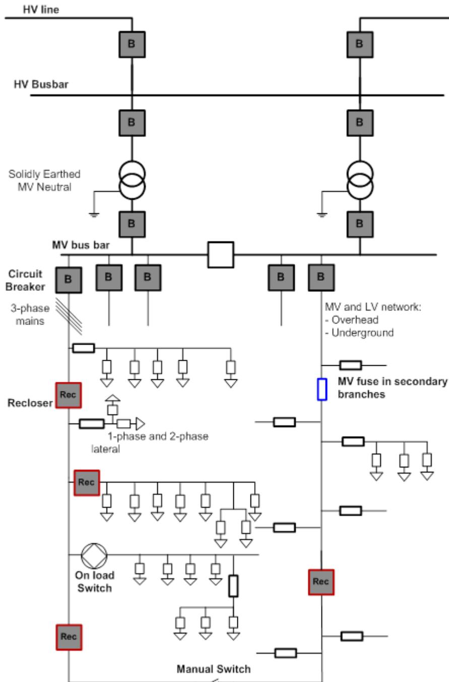
Figure 7: Power delivery overview - MV network model adopted by South American DSOs
