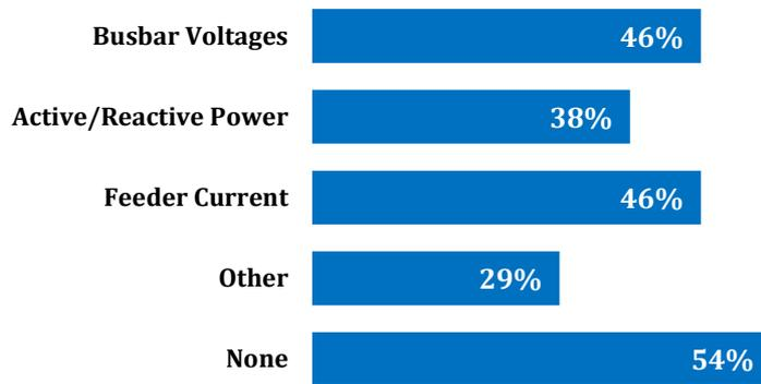
Figure 6 - Monitored System States at MV/LV Substations
