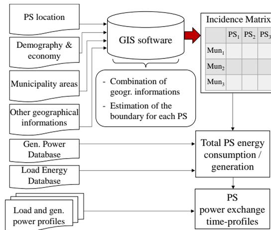
**Figure 26 - Conceptual scheme to obtain the power exchange profiles for a given DN from different datasets.**
