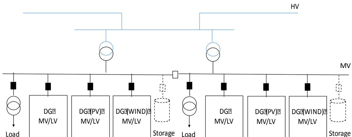
**Figure 21 – Aggregation at HV/MV substation**
