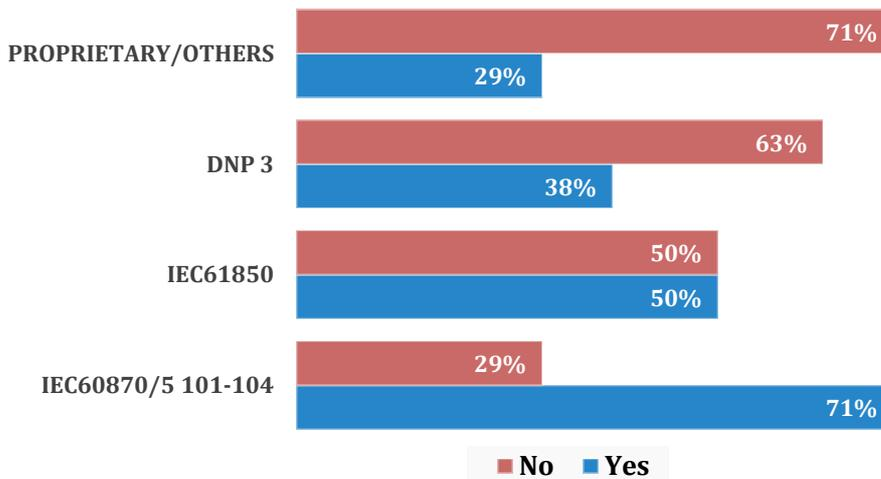
**Figure 15 - Type of Communication Protocol Most Implemented**
