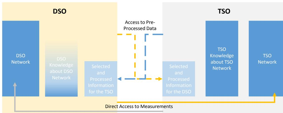
**Figure 22 - High-Level View on TSO-DSO Information Exchange**
