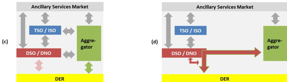
**Figure 24 - Examples schemes for physical access to DER in DSO systems**
