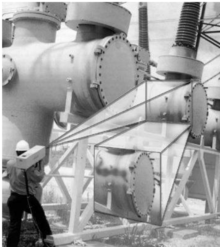
Figure 4-16: Gas leak inspection of a SF 6 CB with laser system [Keith2000]
