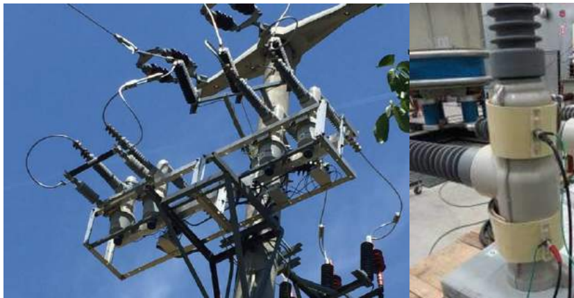
Figure 3-24: On-line PD measurement on 27kV solid dielectric insulation recloser [Uzelac2015]
