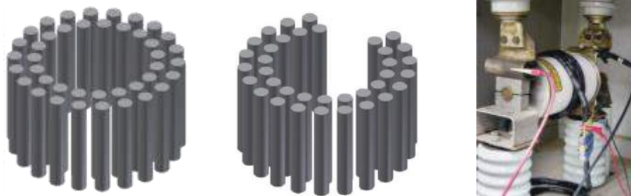
Figure 3-43: Left: Permanent magnet arrangements as two exemplary devices for the generation of the magnetostatic field [Eichhoff2014a], Right: Flexible coil system for the generation of the magnetostatic field [Cadick2014b]
