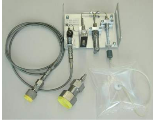
Figure 3-20: Detector tube and sampling arrangement
