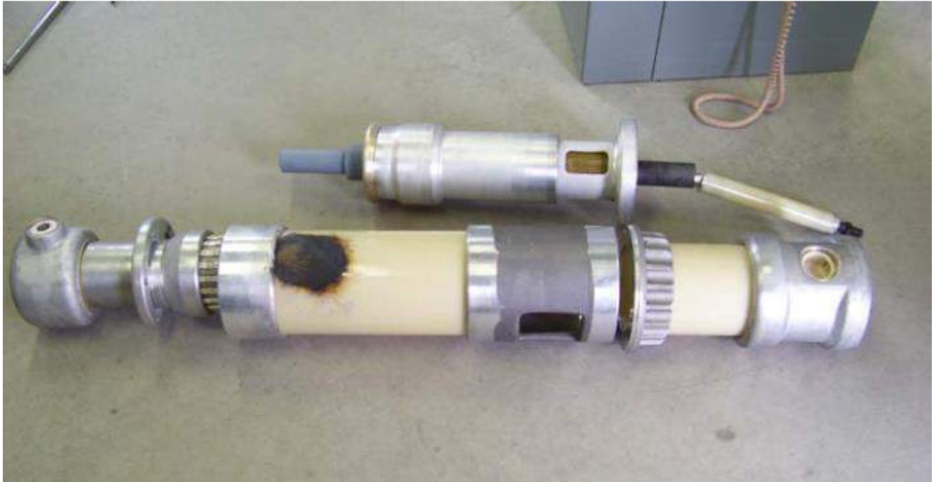
Figure 4-23: Signs of flashover on a circuit breaker
