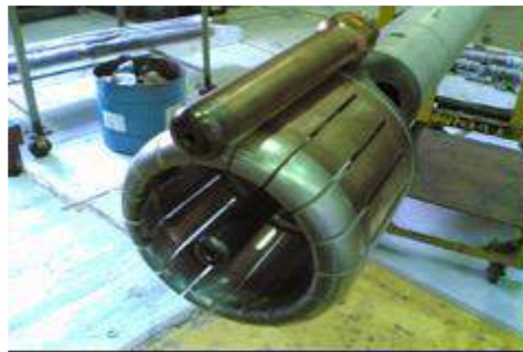
Figure 3-13: Wrong assembly; 31.5 kA arcing contact instead of 40 kA arcing contact used [Sodha2012]
