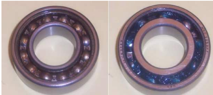
Figure 4-27: Lacking of lubrication of a trip-latch bearing (left-hand side) [Larson2009]
