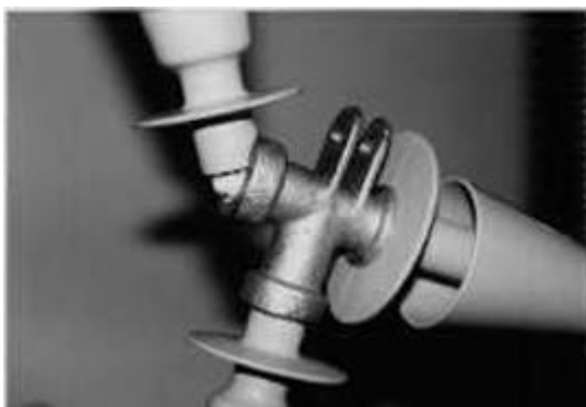
Figure 9 . Flexural load breaking test (Trail A: Bell type)
