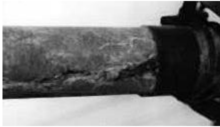
Figure 5. Tracking of EPR specimen (4.5 years)
