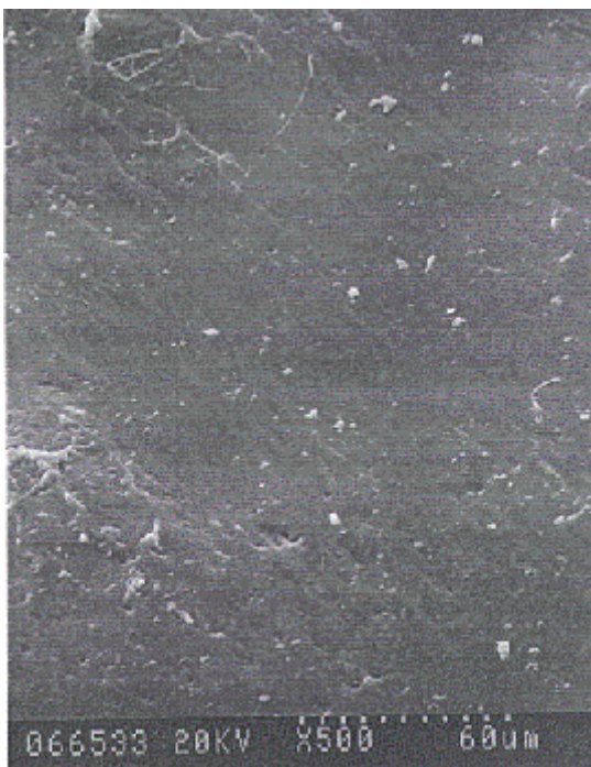
Figure 2c SEM picture of the surface of an unexposed specimen
