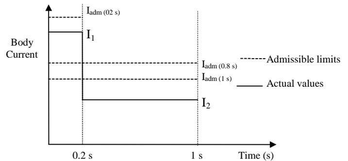
Figure 6: Actual and admissible body currents during a fault
