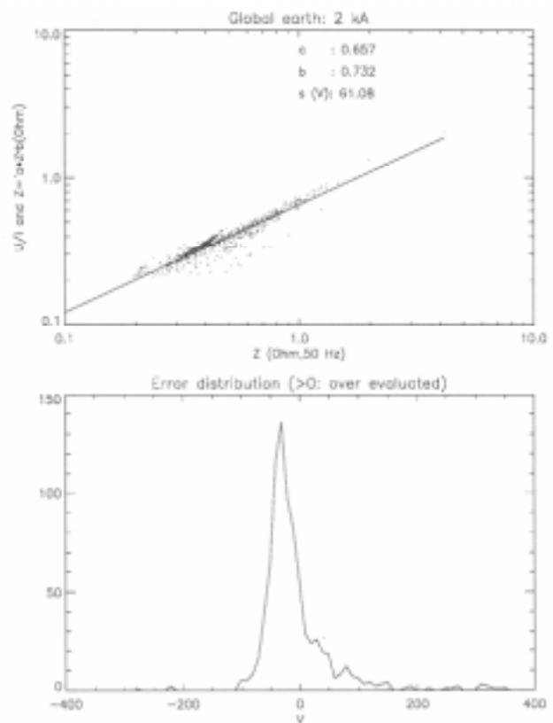
Figure 3a: Correlations between  $U/I$  and  $Z$  (at 50 Hz)
