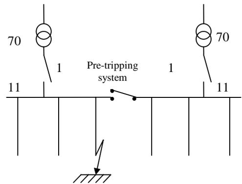
Figure 5: Pre-tripping in MV networks
