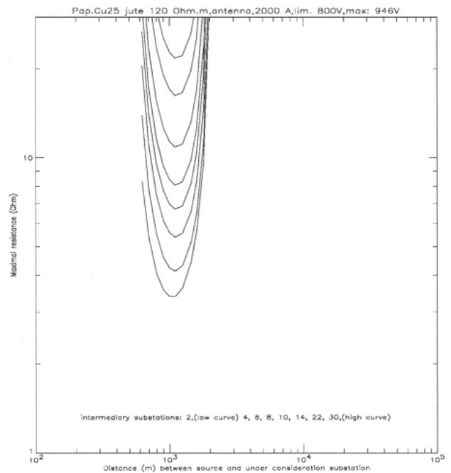
Figure 1: Maximum allowed earth resistance in a MV underground network (Paper jute Cu  $25^2$ )
