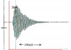
Such bursts of current may range from just a few to several hundred Amperes but typically only last a few tens of milliseconds and are far too small and short to cause operation of conventional main overcurrent protection.
