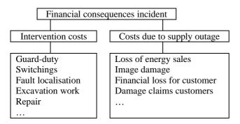
A severe incident on a network component will always result in an intervention. The most significant costs are imputable to intervention of the guard-duty, switchings, fault localisation, excavation work, repair and material costs. The sum of these partial costs represents the total intervention costs.
