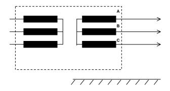
The current appearing during a ground fault can only circulate through the capacities between the phase conductor and the ground. It is of low amplitude. Under single-phase fault conditions the voltages of the healthy phases are increased to the phase-to-phase voltage of the network. This has to be taken into account in the definition of the insulation properties of the network.
