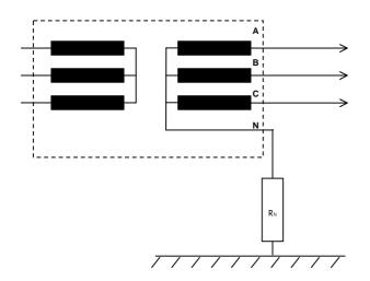
The limiting resistor is inserted between the MV neutral of the HV/MV transformer and the ground of the substation.
