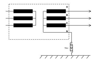
The limiting impedance can be inserted between the MV neutral of the HV/MV transformer of the substation and the ground of the substation. To be independent from the presence of a MV neutral point of the HV/MV transformer of the substation, it is possible to create an artificial neutral point.
