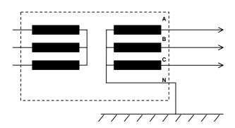
The insulation level of networks without distributed neutral remains nearly equal to the line-to-earth voltage, the ground potential rise in the proximity of the ground fault are conditioned by the quality of the earthing terminals which must have a very low resistance.
