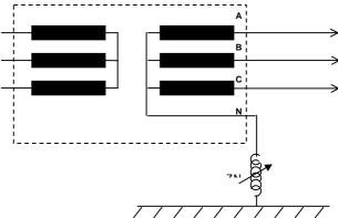
The compensating coils are variable limiting impedances.
