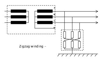
This mode of grounding is employed on the MV distribution networks in France since the years 1950. The specification HN 52-S50 of EDF, the national utility of France, thus specified two types of neutral reactors (zigzag winding) for the 5,5kv-10kv-15kv-20kv-30kv networks. A 300 A reactive fault current version is destined for the rural networks with overhead lines, whereas the 1000 A version is gauged for urban networks mainly made of underground cables.
