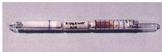
Figure 6. Colour change in Dräger Tube – Sludged switchgear oil
