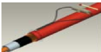
Figure 1 – Faraday current sensor
