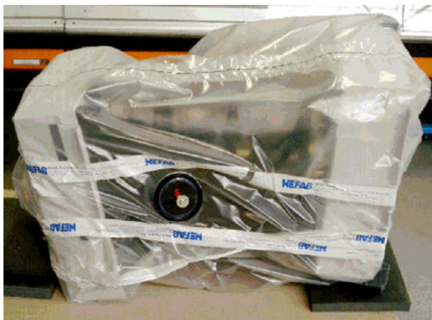
Tightness test: body to be tested in a plastic bag equipped with a measuring valve.
