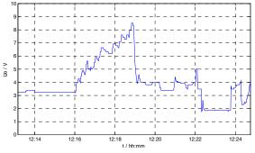
Fig. 9: Disturbed U<sub>0</sub> without switch-operation or coil movement
