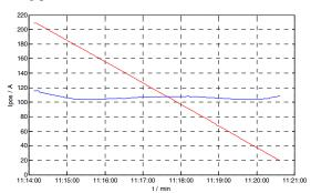
Fig. 8: Estimated resonance point during coil movement
