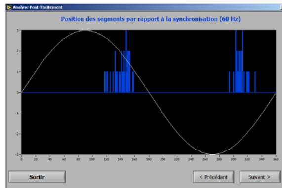
Figure 4. Phase resolved detection for the defective cable joints shows that PD activity shifts by 90°. Most PD pulses occurred in the 2nd and 4th quadrants [1].
