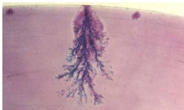
Figure 6. Example of “vented” water tree in XLPE
