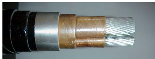
Figure 1. Three core PILC cable with aluminium conductor
