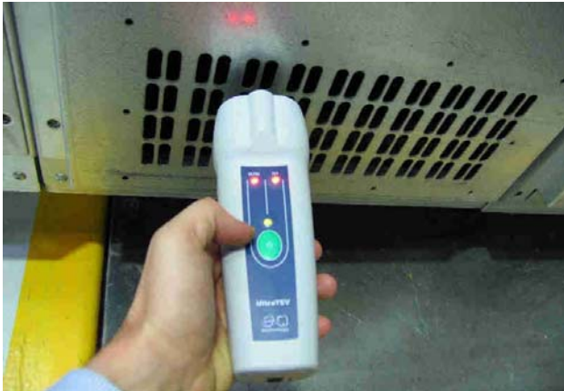
Fig 4. Ultrasonic (left led) and TEV (right led) detection active
