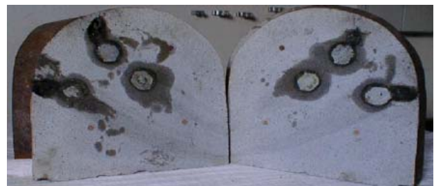
Figure 1: Cross section of a weak nekaldiet joint
