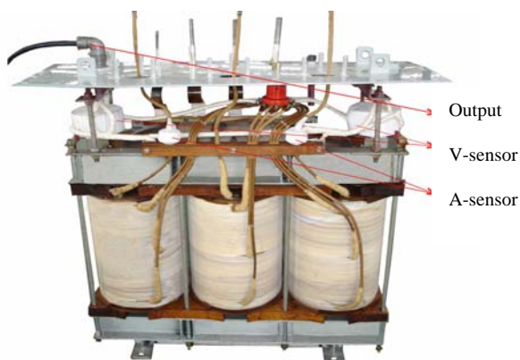
Figure 5 The picture of assembled transformer with embedded sensors
