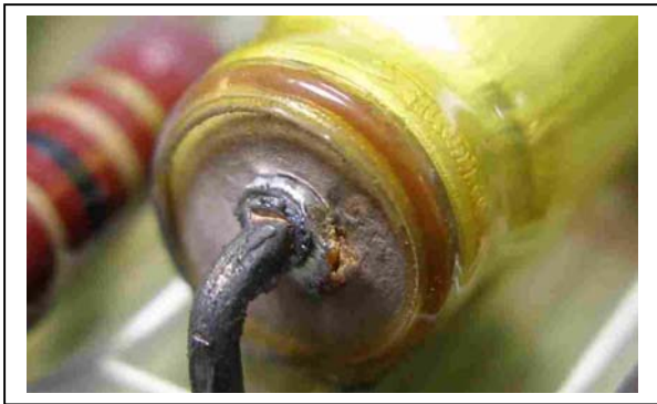
Figure 1: damaged chemical capacitor
