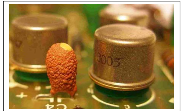
Figure 5: aging tantalum capacitor placed in a severe thermal environment
