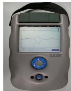
Figure 1: IFL-1000 Intelligent Fault Locator [10]
