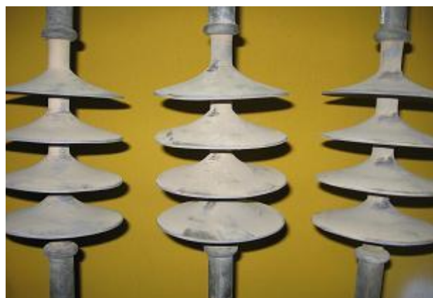
Figure 1. SIR specimen insulators No.2, No.3 and No.4.
