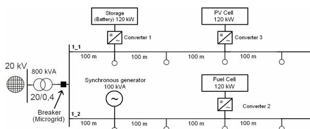
Figure 1. Studied urban LV network based microgrid.
