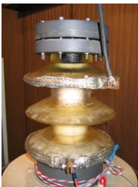
Figure 2: probe insulator with condensed moisture Figure 3: Atmospheric condition measuring subsystem
