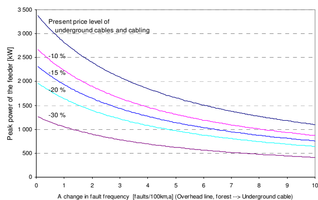
Fig. 2. Economical limits (kW) for underground cabling depending of the fault frequency development and the price of cabling. A change in fault frequency indices estimated improvement in reliability when OH lines are replaced with UG cables. For instance 0 indices that there are as many permanent faults in the UG cable as in the OH line network, whereas 10 means that all the 10 faults can be avoided in the UG cable network. Reconnection time is 1 h.
