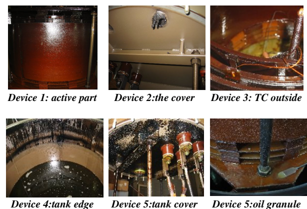
Fig 4 Images of the internal part of the devices at the end of cycle
