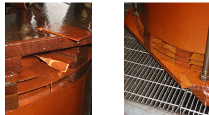
Fig.2 Sampling of pressboard from the upper and lower angle ring of the active part of a device
