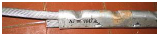
Fig. 4: Photograph of a joint for Al/Fe 70/12, Type 1
