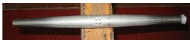
Fig. 6: Photograph of a joint for Al/Fe 70/12, Type 2
