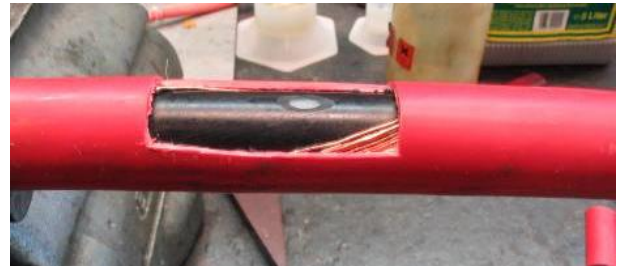
Fig. 4: Artificial defect (damage of semicon layer)
