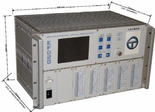
Fig.1: Integrated protection System
