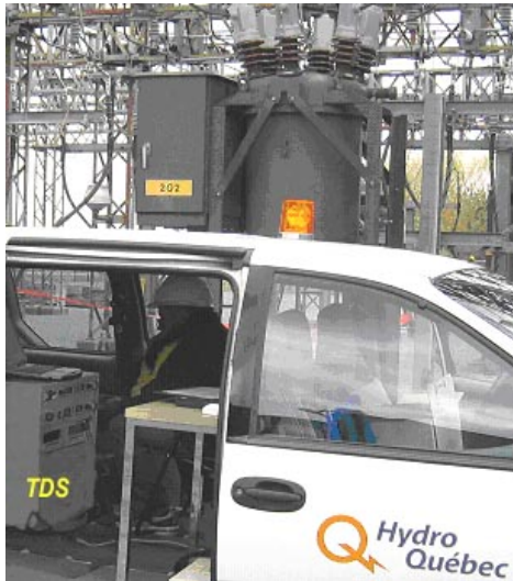
Figure 2: TDS device installed in a small vehicle for field measurements
