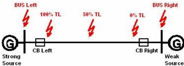
Figure 2 – Faults Simulation System modeling with the faults simulations positions
