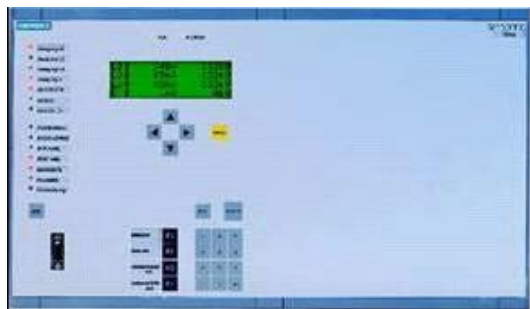
Figure 5 – Numeric Distance Protective Relay 7SA612
