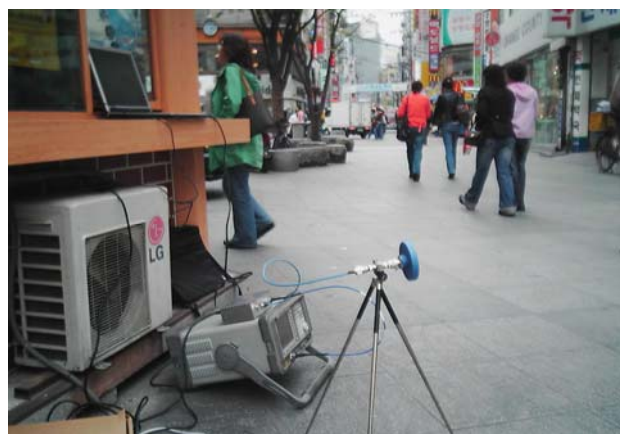
Fig. 5. The external noise measurement at site
