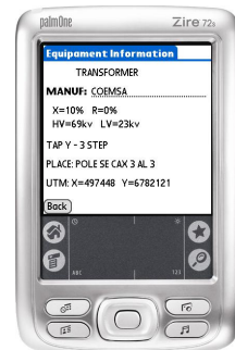
Figure 11 - Results of transformer database query.
