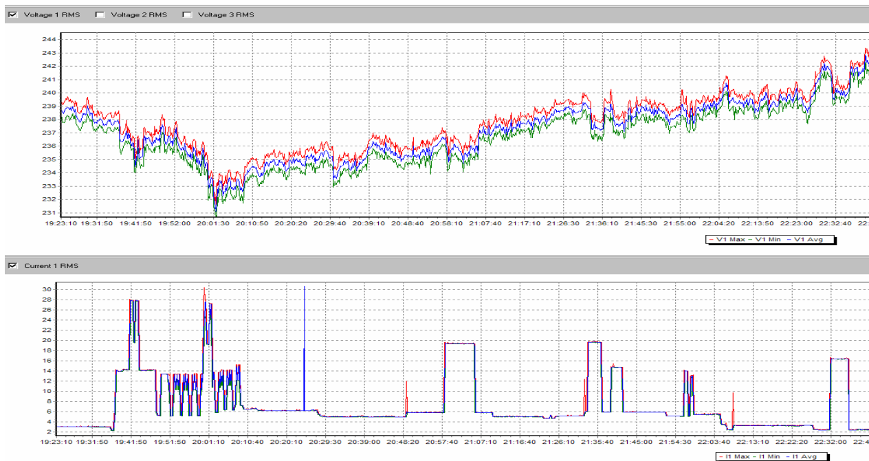
Fig 2: Voltage and current of a single phase household supply; 10-second measurements over 3 hours
