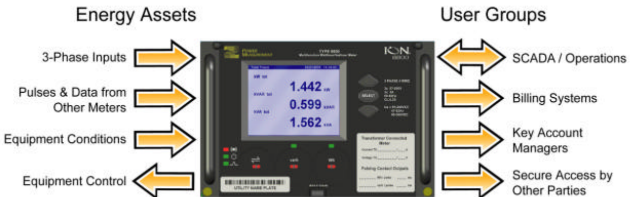
Figure 3 Information flow from Smarter Meters
