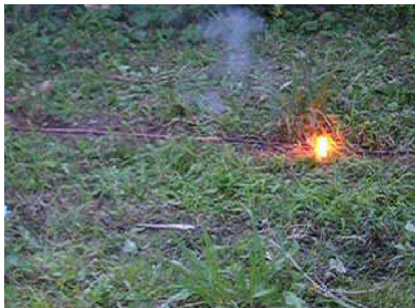
Fig. 8. Validation of HIF Detect™ on soil.
