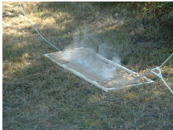
Fig. 6. Validation of HIF Detect TM on sand.
