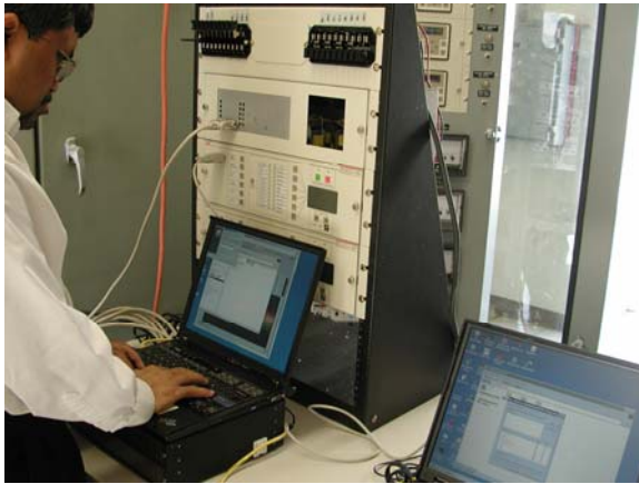
Fig. 4. HIF Detect TM equipped IEDs and data collection system.
