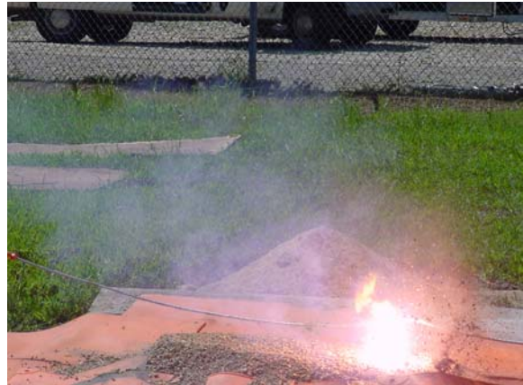
Fig. 5. Validation of HIF Detect TM on gravel.
