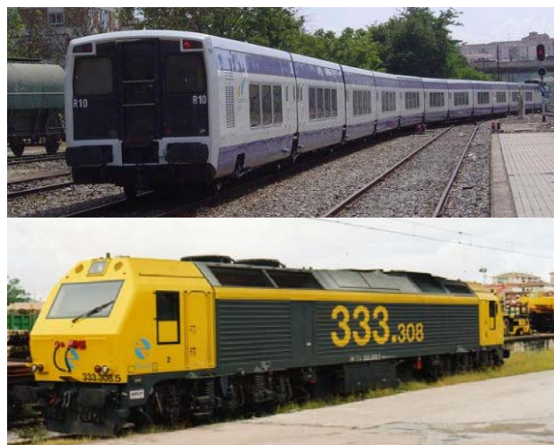
Figure 1. Talgo IV coaches and diesel-electric locomotive used for haulage.
