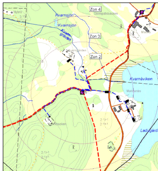
Figure 2. Customer connections in Zone 2 and 3. The LV network is draw with blue broken lines.
