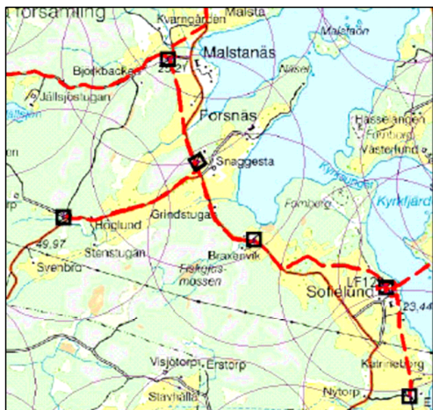
Figure 3. Circles indicating Zone 4 outer boundaries with 1000 m radius from substations. The figure illustrates the zone model's grade of covering the total area.
