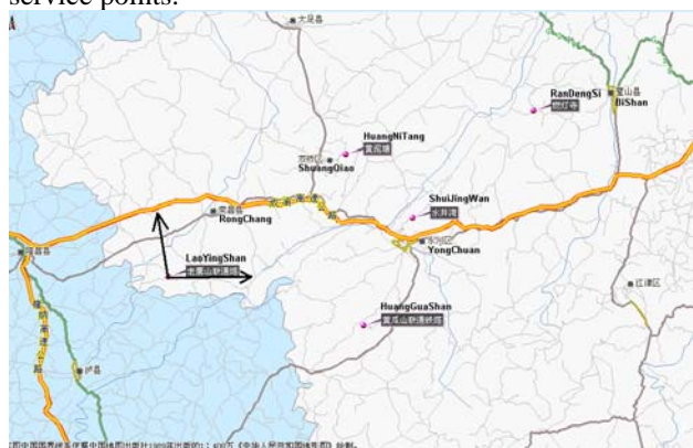
Figure 2. Distribution of base stations in CHONGQING POWER SCDMA communication network(phase I)
