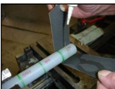
Fig. 4: creation of calibrated defects
