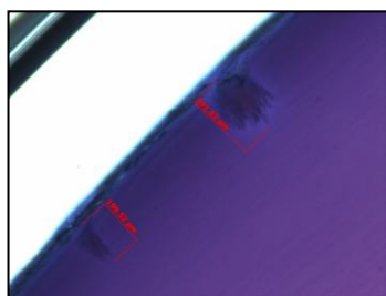
Fig. 7: water trees in sample 1
