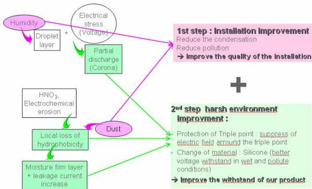
Figure 4- two origins for the degradation
