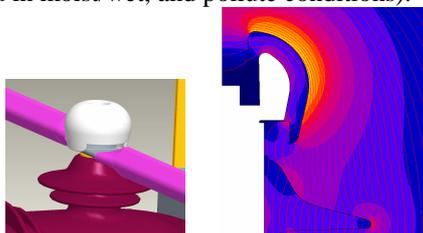
Figure 6- Field distributor for normal offer
