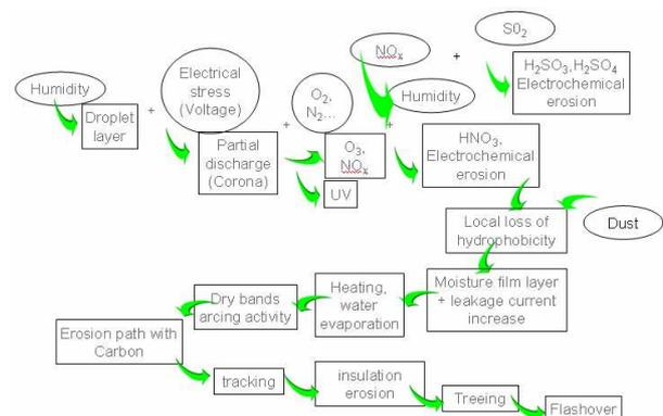
Figure 3- Degradation process
