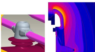
Figure 7- Field distributor with silicone device for triple point protection
