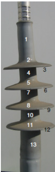
Fig 5: Measuring points of the hydrophobic class spread along the surface of the termination.
