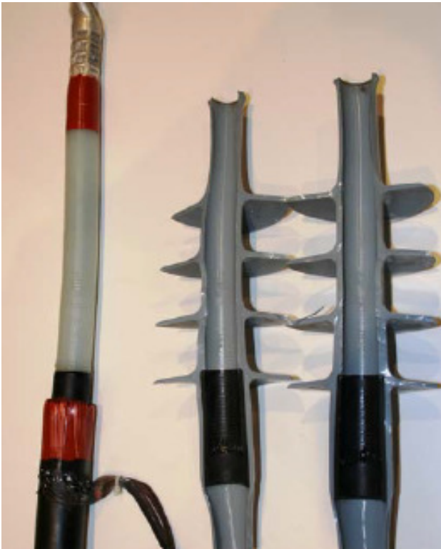
Fig. 6: Overall view of the dismantled termination and the VPE cable.
