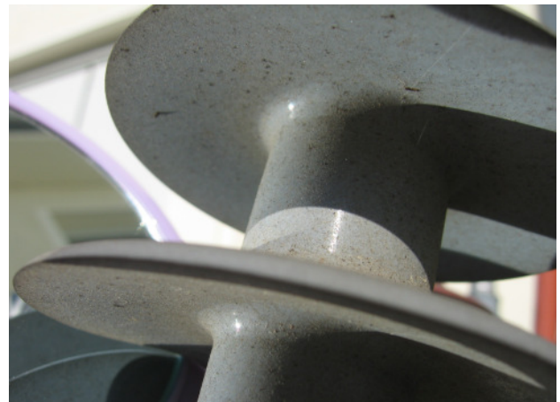
Fig. 3: detailed view of a termination after the long term electric stress.
