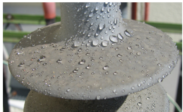
Fig. 4: Termination sprayed with water droplets.
