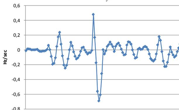
Network configuration allowed testing different combinations of generators. In one of them, only dozens of inverters with the same impedance measurement method were feeding the islanding system. Those inverters failed to detect the islanding situation, probably affected by the interaction between inverters.
