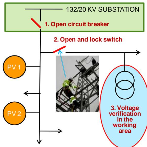
In this case, the workers considered that voltage absence verification in the MV feeder was not necessary. On the one hand, because isolation from voltage sources is a previous step to voltage verification, according to safety legislation in force (see figure 1). On the other hand, because they did not have to work on that place, but on equipment located away from the isolation point.
