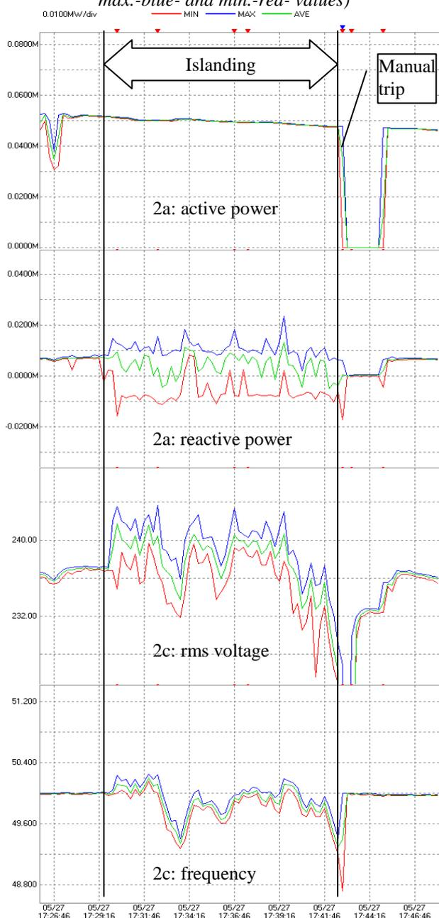
The test process started from a situation in which generation was higher than consumption. To balance roughly the power, some inverters were manually disconnected until the current by the substation MV circuit breaker decreased to a few amperes. Then, the feeder circuit breaker was open. In both cases, the islanding event was reproduced, giving rise to islanding networks of, roughly, 700 kW and 2.5 MW.
