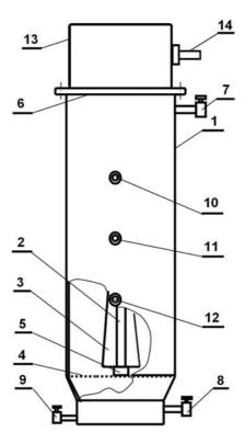
**Figure 1 -** Universal regeneration cartridge 1- external tube, 2 – center conductor, 3 – ribs for redistribution the electromagnetic field, 4 – filtering mesh, 5 – insulator, 6 – flange, 7-9 – oil and air gates, 10-12 – thermometer gates, 13 - device for electric matching, 14 – gate for UHF energy.
