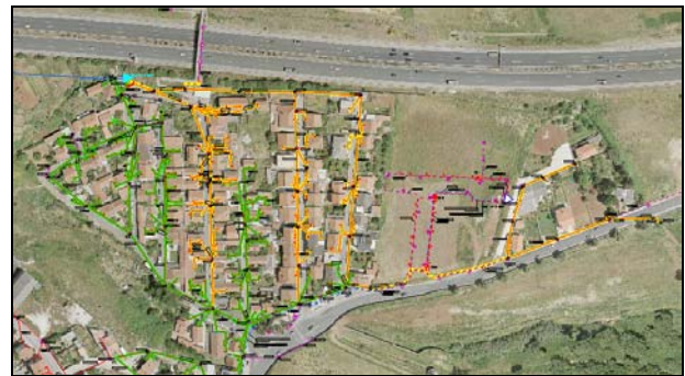
Figure 4. 250 kVA PT feeders in a low consumption suburban residential area
