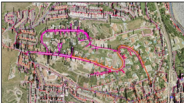
Figure 7. 400 kVA PT feeders in a high consumption suburban residential area
