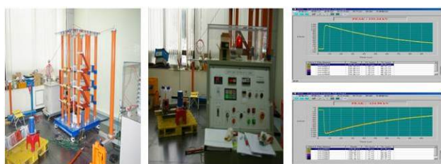
Figure 7 AC/Impulse withstand voltage test
