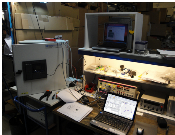
Figure 2: Testing the under-voltage dependent directional reactive power relays
