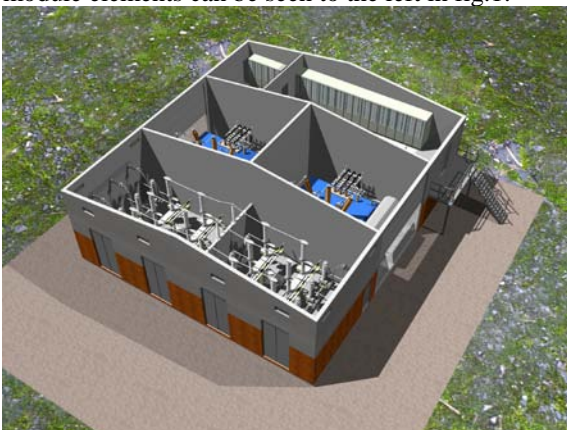
Fig. 2: Layout of Bäckelund substation
