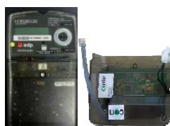
Fig 4- Energy Box and PLC communication module
