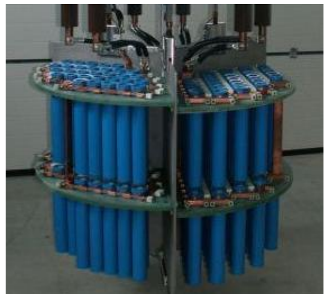
Figure 4: Internal construction of the SFCL for trial 2
